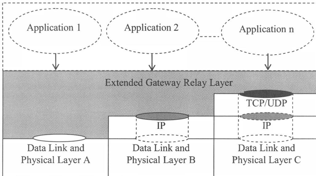
**Fig. 5. Extended Gateway architecture**
