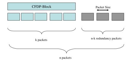
Fig. 1. CFDP-UE-RSE Creation of Redundancy Packets.
