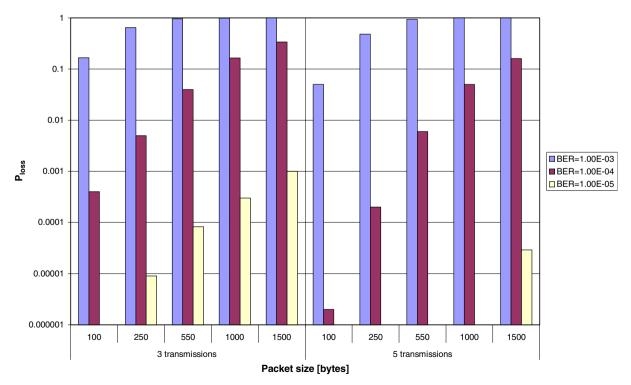
Fig. 6.  $P_{\text{loss}}$ , 3 and 5 transmissions, CFDP-UE-RT.
