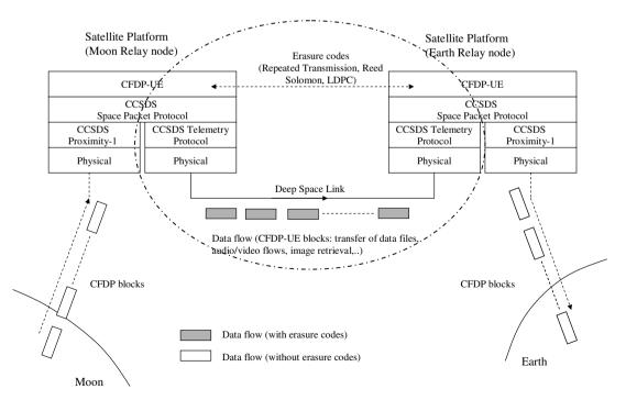
Fig. 4. The testbed and the CCSDS protocol architecture.
