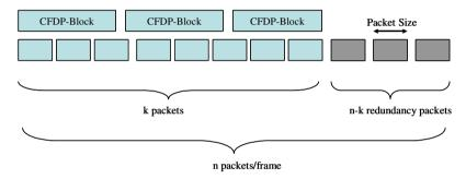
Fig. 2. CFDP-UE-LDPC Creation of Redundancy Packets.
