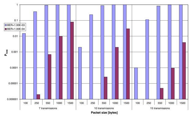
Fig. 7. Ploss, 7, 10 and 15 transmissions, CFDP-UE-RT.
