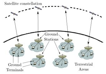
Fig. 1: Nanosatellite constellation application scenario
