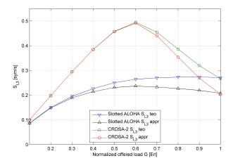
Fig. 4. Layer 3 throughput comparison between exact and approximated  $P_{succ-L3}$  and with  $f_X(x)=e^{-x}$
