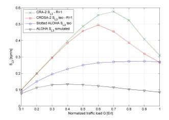
Fig. 3. Layer 3 throughput simulations with  $f_X(x) = e^{-x}$
